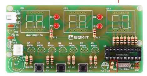
Step 13:Install 1pcs 100uF/16V Electrolytic Capacitor at C6.Pay attention to the installation direction and the shorter pin is negative pins.
